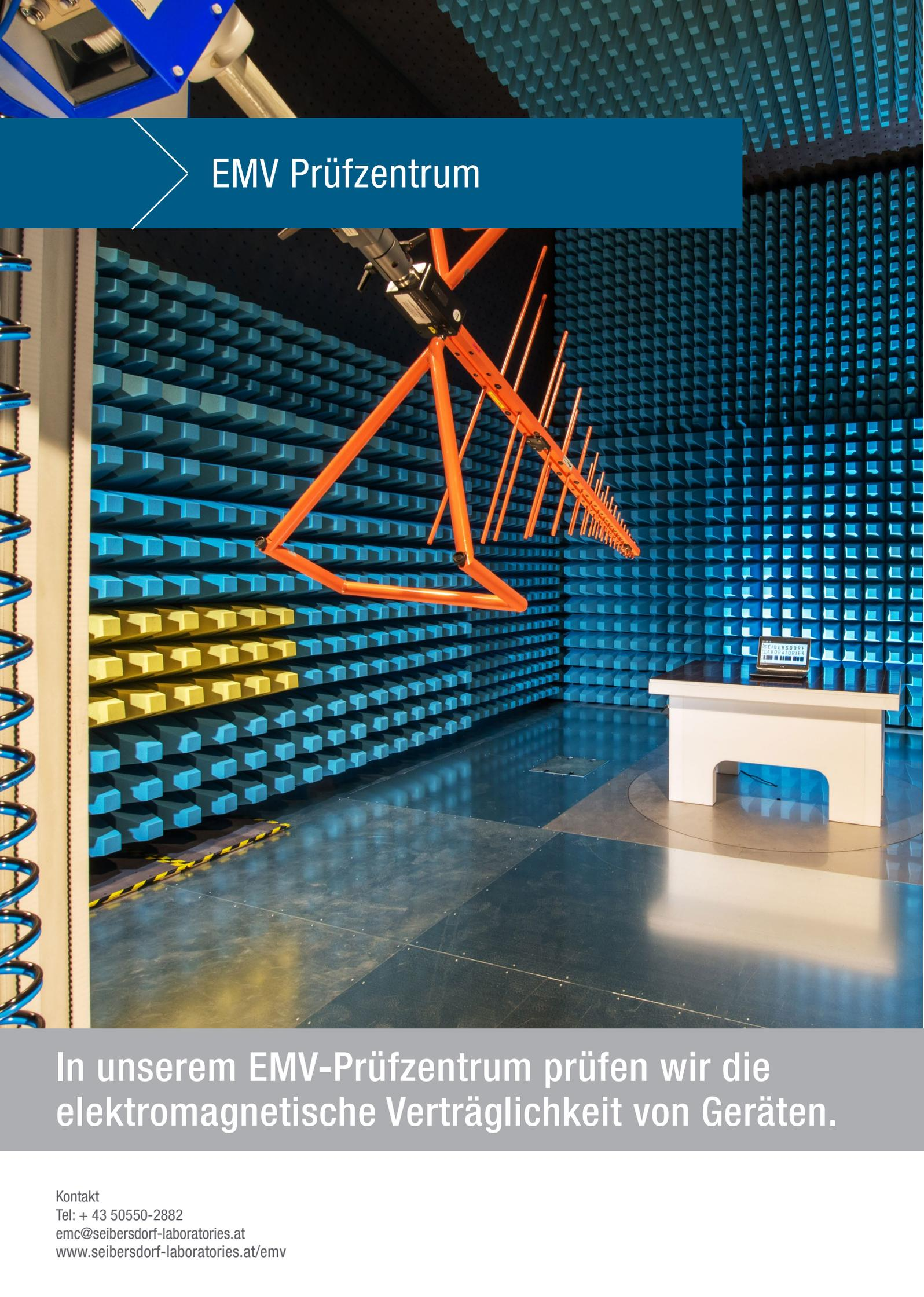
The image shows an anechoic chamber with blue pyramidal absorbers on the walls and ceiling. A yellow mechanical arm is suspended from the ceiling, holding a probe. In the foreground, there is a white table with a laptop on it. The laptop screen displays the logo for 'SEIBERSDORF LABORATORIES' and the text 'EMV IN SEIBERSDORF'.
